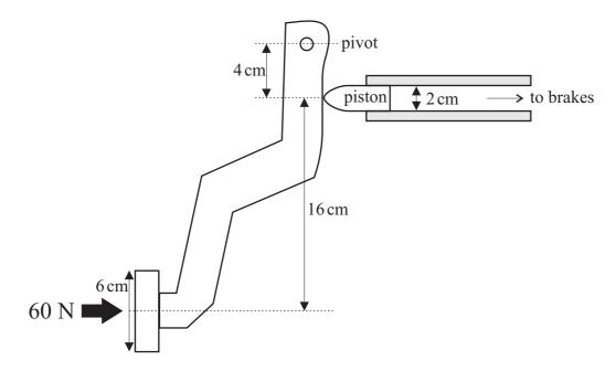
A driver applies a force of 60N to the pedal. What force is applied to the piston?
